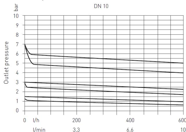
Characteristics are valid for a flow rate of 2 m/s
